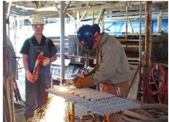
Welding with fire control
