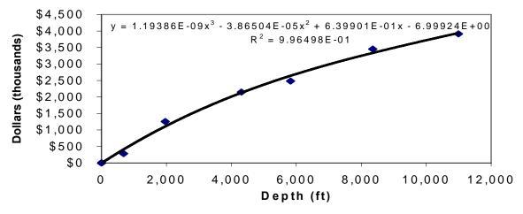
Figure 3. Average depth versus median cost from Table 1 for geothermal wells in Central America and the Azores from 1997-2000 (from Table 1 data).
