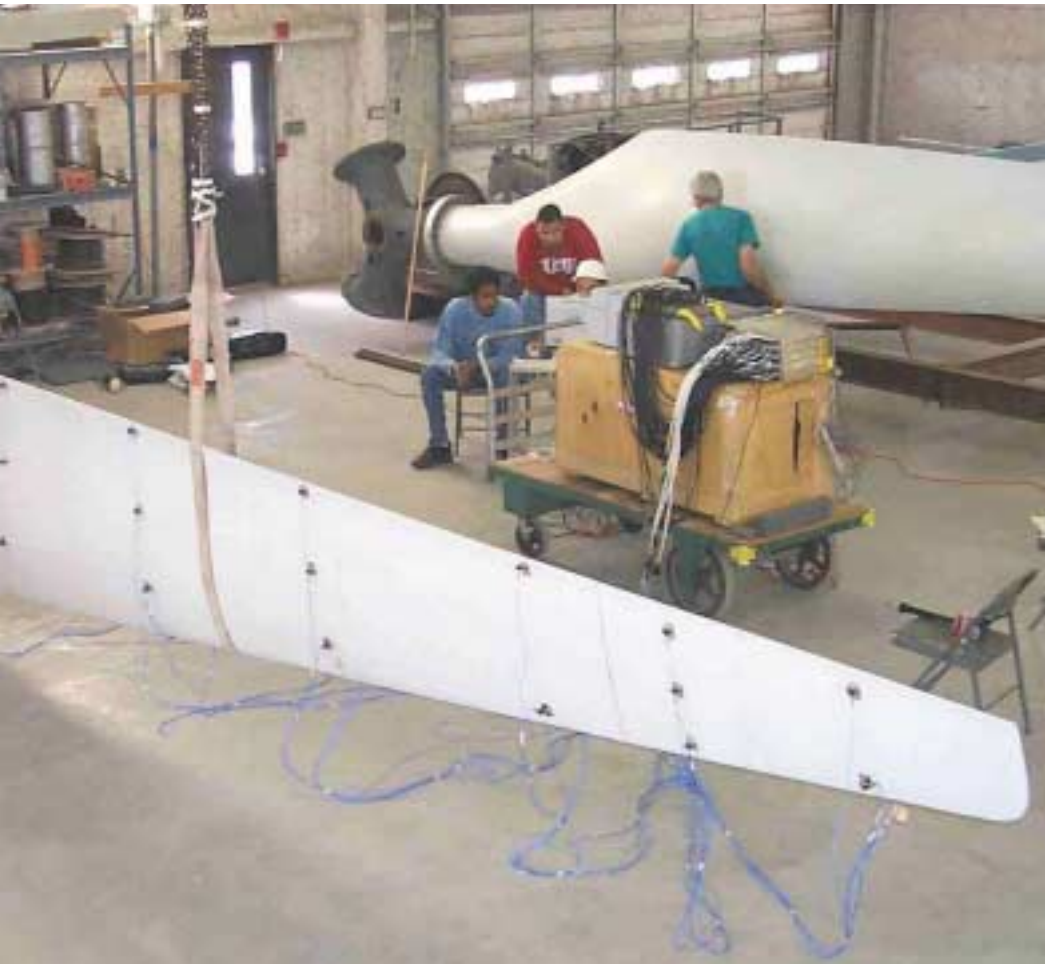
Left to right: Modal testing provides researchers with information about the wind turbine's physical properties as part of the Long-Term Inflow and Structural Testing National Laboratories, Albuquerque, New Mexico
