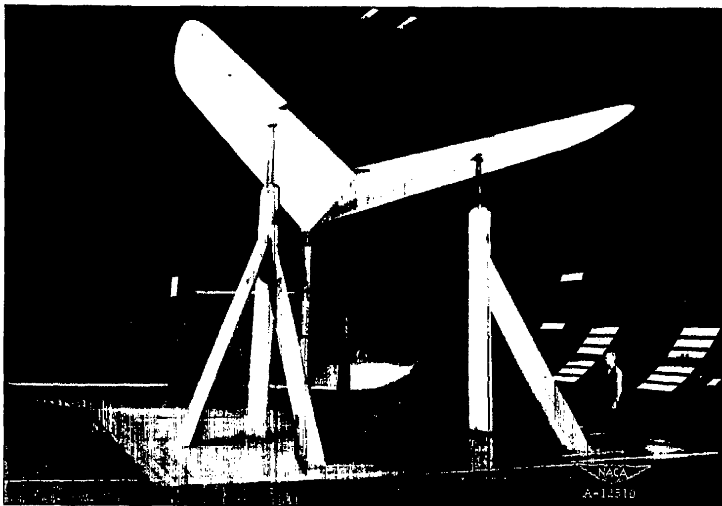
Figure 2.- The 45^\circ swept-forward wing in the Ames 40- by 80-foot wind tunnel. Inboard one-half-span leading-edge flap deflected down.
