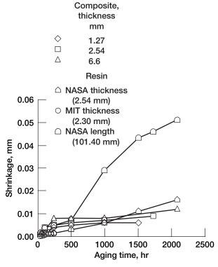
Figure 14.—Shrinkage of PMR–15 neat resin and composites during aging at 316  $^{\circ}$ C.
