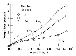
Figure 8.—Weight loss fraction of PMR-15 neat resin specimens as function of aging time at 225 °C. Weight gain mechanisms predominate during first 200 hr of aging (ref. 2).
