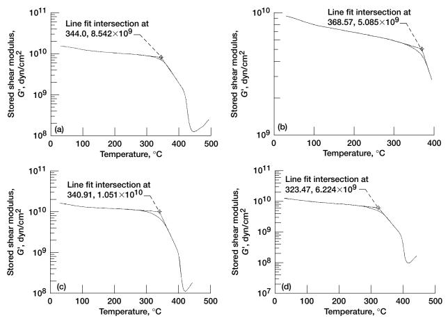
Figure 3.—Dynamic shear modulus measurements of PMR-15 neat resin specimens after aging. (a) No aging. (b) 316  $^{\circ}$ C for 2534 hr. (c) 260  $^{\circ}$ C for 4312 hr. (d) 204  $^{\circ}$ C for 4200 hr.
