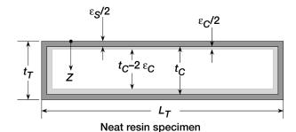
Figure 16.—Dimension notations for equations (4) to (6) describing shrinkage values.  $L_T$ , original length;  $t_C$ , core thickness;  $t_T$ , original thickness;  $\epsilon_C$ , core shrinkage;  $\epsilon_S$ , surface layer shrinkage; Z, distance from center of specimen.
