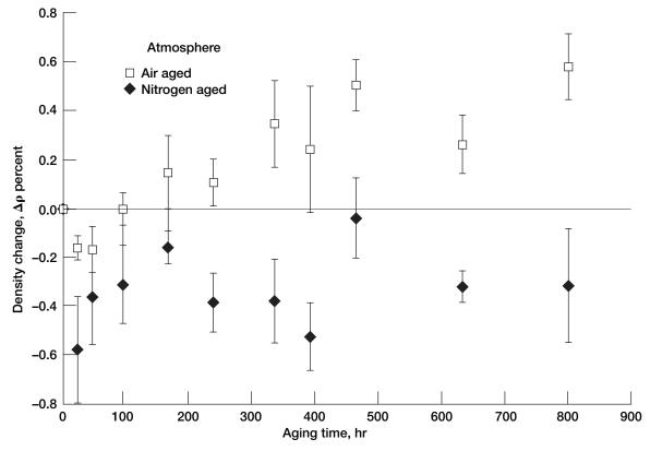
Figure 2.—Density changes of PMR-15 neat resin specimens during aging in air and nitrogen at 316  $^{\circ}$ C (ref. 5).
