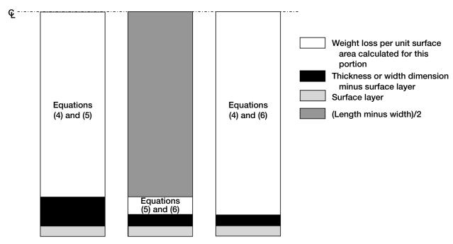
Figure 17.—Specimen areas described by equations (4) to (6).
