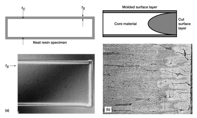
Figure 10.—Development of oxidized surface layer on neat resin and T650–35/PMR–15 composite after aging in air at elevated temperatures. (a) PMR–15 neat resin oxidized surface layer. Surface layer thickness,  $t_{\rm S}$ ; core thickness,  $t_{\rm C}$  (ref. 7). (b) T650–35 composite oxidized surface layer.
