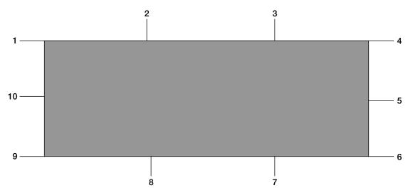
Figure 1.—Marked index position for dimensional measurements. Total measurements made: 10 thicknesses, 4 widths, 3 lengths (1–4; 4–6; 6–9; 9–1; 7–3; 8–2; 10–5).
