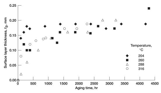
Figure 11.—Development of PMR-15 neat resin surface layer as function of aging time and temperature.
