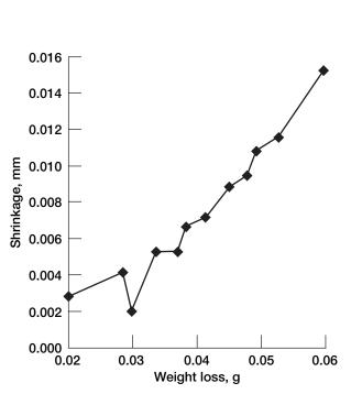
Figure 13.—Shrinkage of PMR-15 neat resin specimen length as function of specimen weight loss during aging at 316 °C.
