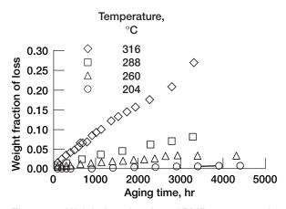
Figure 5.—Weight loss fraction of PMR-15 neat resin specimens as function of aging time and temperature.
