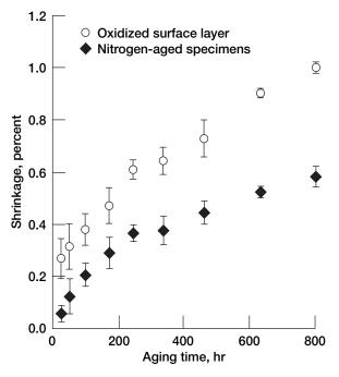
Figure 15.—Shrinkage of PMR–15 neat resin specimens aged in air and nitrogen at 316  $^{\circ}$ C as function of aging time (ref. 6).
