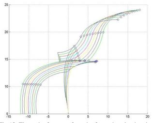
Fig.13. The path of center of gravity for various bogies size (all dimensions are in cm)
