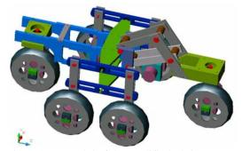
Fig.3. CAD model of the modified Shrimp Rover
