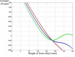
Fig.15. Torque needed for climbing for three different springs
