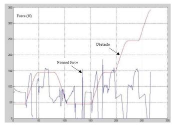
Fig. 16. Back wheel force diagram during obstacle crossing
