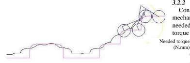
Fig.12. The path of C.G on the experimental stairs
