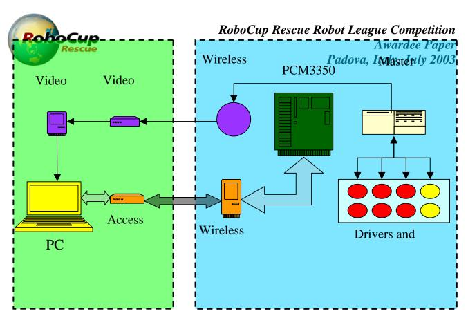
Rescue Station Fig. 19. The communications and control units
