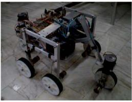
Fig.1. Alpha prototype of the Shrimp Rover
