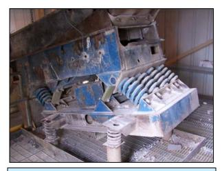
Vibrating screens can generate over 105 decibels. Grommets and rubber mounts can greatly reduce the vibration-generated noise.
