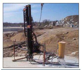
Drill noise is generated by the pneumatics and engine exhaust, as well as the drill steel. Highwalls can reflect and amplify the noise levels.
