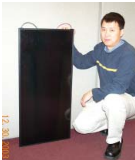
Note added in proof: The above photo shows a recently-made, full-size, hybrid CIGS module
