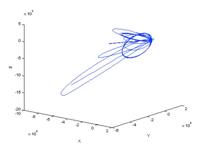
Trajectory of the Cassini vehicle in the J2000 frame, for June 20, 2004 to Dec 1, 2005
