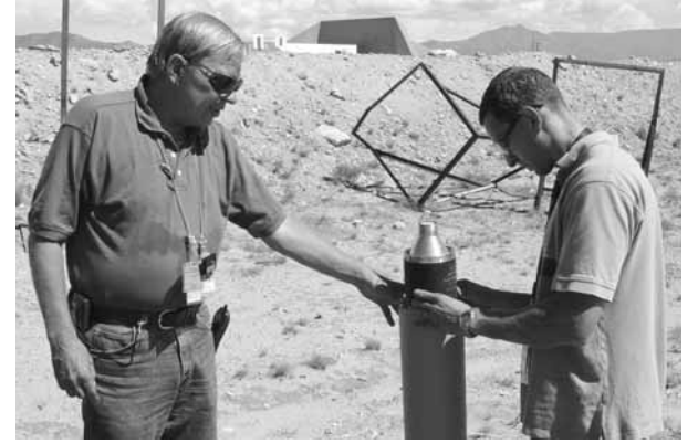
DAVID PAUL, left, and Brian Melof prepare a shaped charge for a test. David is spooling out the shock tube, which is used to set off the explosive shaped charge for the test.
