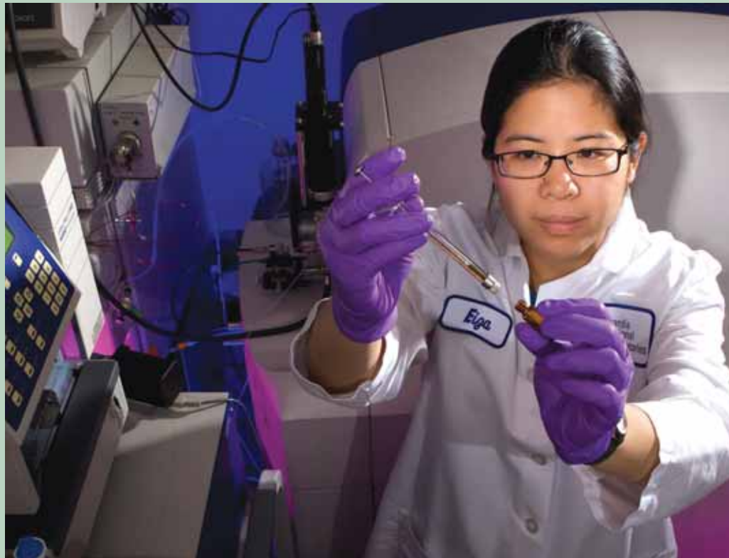
GREEN GOLD — Eizadora Yu injects a sample of extracted algal oil into a mass spectrometer for analysis of molecular species. (Photo by Randy Wong)
