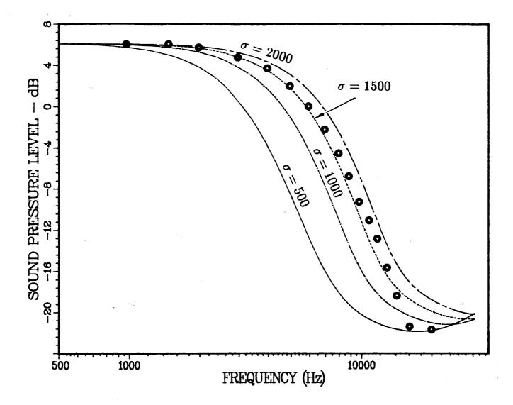
Figure 1. Typical results for determination of flow resistivity  $\sigma$  of carpet material on plywood. Shown are predicted and the measured SPL-versus-f curves for sound propagating over carpet; the source height is two centimeters and the receiver height is 0.3 cm; the horizontal separation distance between source and receiver is 80 cm. From the data shown it is inferred that  $\sigma$  is approximatey 1500 Rayls cgs.
