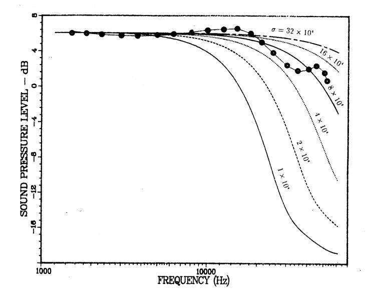
Figure 2. Typical results for determination of flow resistivity  $\sigma$  of plywood. Shown are predicted and the measured SPL-versus-f curves for sound propagating over carpet; the source height is two centimeters and the receiver height is 0.3 cm; the horizontal separation distance between source and receiver is 100 cm. From the data shown it is inferred that  $\sigma$ is approximatey 80,000 Rayls cgs.
