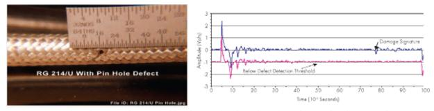
Figure 4. PASD Waveforms from a Test of a Coaxial Cable with a Pin-Hole Defect in the Insulation that Extends to the Inner Conductor.
