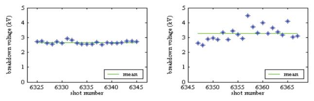
Figure 5. (Left) Example slow-rising, low-energy, DC breakdown voltages for multiple insulation samples. The samples broke down at an average of  $2.8 \pm 0.2 \text{ kV}$ . (Right) When exposed to slowly rising DC after the application of the PASD pulse, the average breakdown voltages remained the same or actually increased. This is a common high-voltage conditioning phenomenon.
