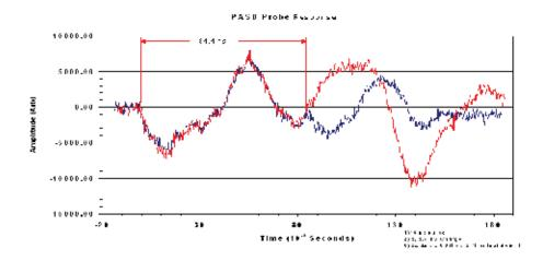
Figure 7. PASD probe waveforms for an insulation chafe defect (DT-1). The PASD waveforms separate at 84.4 ns. This implies that the defect was located at approximately 2.7 m (8.8 ft) from the injection end of the harness. The actual location of the defect was at 2.4 m (8.0 ft).
