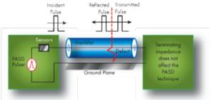
Figure 3. PASD Diagnostic Concept for Locating Defects in Electrical Wiring Systems. (A Single Conductor is Shown Under Test.)
