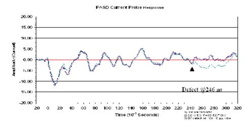
Figure 8. PASD waveforms from a test of a 3-m (100-ft) wire harness with an insulation defect at 24 m (80 ft). The two waveforms deviate at the location of the defect, 246 ns down the line. The variations in the waveforms are caused by a varying impedance profile down the harness. The nature of impedance variations is not important, as PASD uses a differencing technique to locate the defect.
