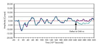
Figure 8. PASD Waveforms from a Test of a 100 Foot Wire Harness with an Insulation Defect at 80 Feet.
