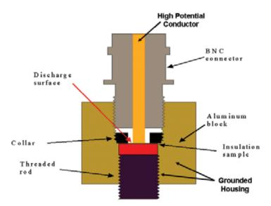
Figure 3. Test fixture used during flashover experiments. Eight-millimeter diameter insulation samples, shown in red, were inserted into the center of the figure. Breakdown occurs on the sample surface between the high potential conductor, which passes down through the BNC connector, and the grounded outer housing at the collar.
