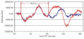
Figure 7. PASD Probe Waveforms for an Insulation Chafe Defect.
