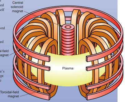
In a tokamak, magnetic fields from surrounding magnets confine a plasma fuel of hot, ionized gas within a hollow, doughnutshaped vacuum chamber. National Laboratory. In fact, the collaboration is the biggest user of NERSC facilities. The current simulations typically require from 10 to 20 hours to complete using NERSC's most powerful machines.
