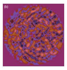
The UCAN code, developed by Livermore collaborators at the University of California at Los Angeles, produced these two images of tokamak plasmas. (a) Early in the development of the microturbulence, smallamplitude, radially elongated turbulent eddies form. (b) Fully developed microturbulence exhibits smaller, disordered structures.
