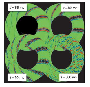
This simulation, done by Livermore collaborator General Atomics of San Diego, California, with the GYRO code, shows a cross section of a tokamak over time (*t*) in microseconds (ms). The color contours indicate microturbulent fluctuations in the plasma density. The center sections have been removed to facilitate comparison.
