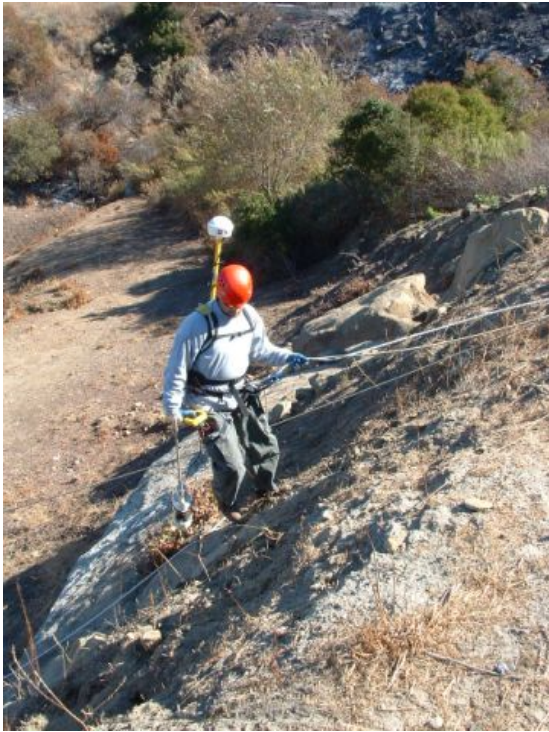
Figure 3.1 – Physical Restraint System for Slope Surveying
