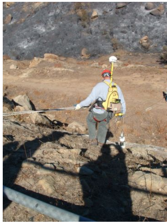
Figure 3.1 – Physical Restraint System for Slope Surveying
