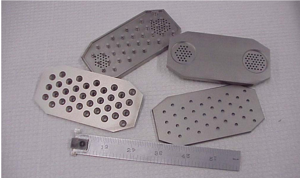
Figure 6. Upper and lower plates of the Flat-Plate Hot Heat Exchanger
