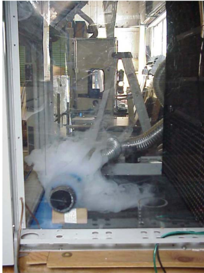
Fig. 3.12.2 Large Smoke containment failure, note smoke outside sash plane in far left of this side view.
