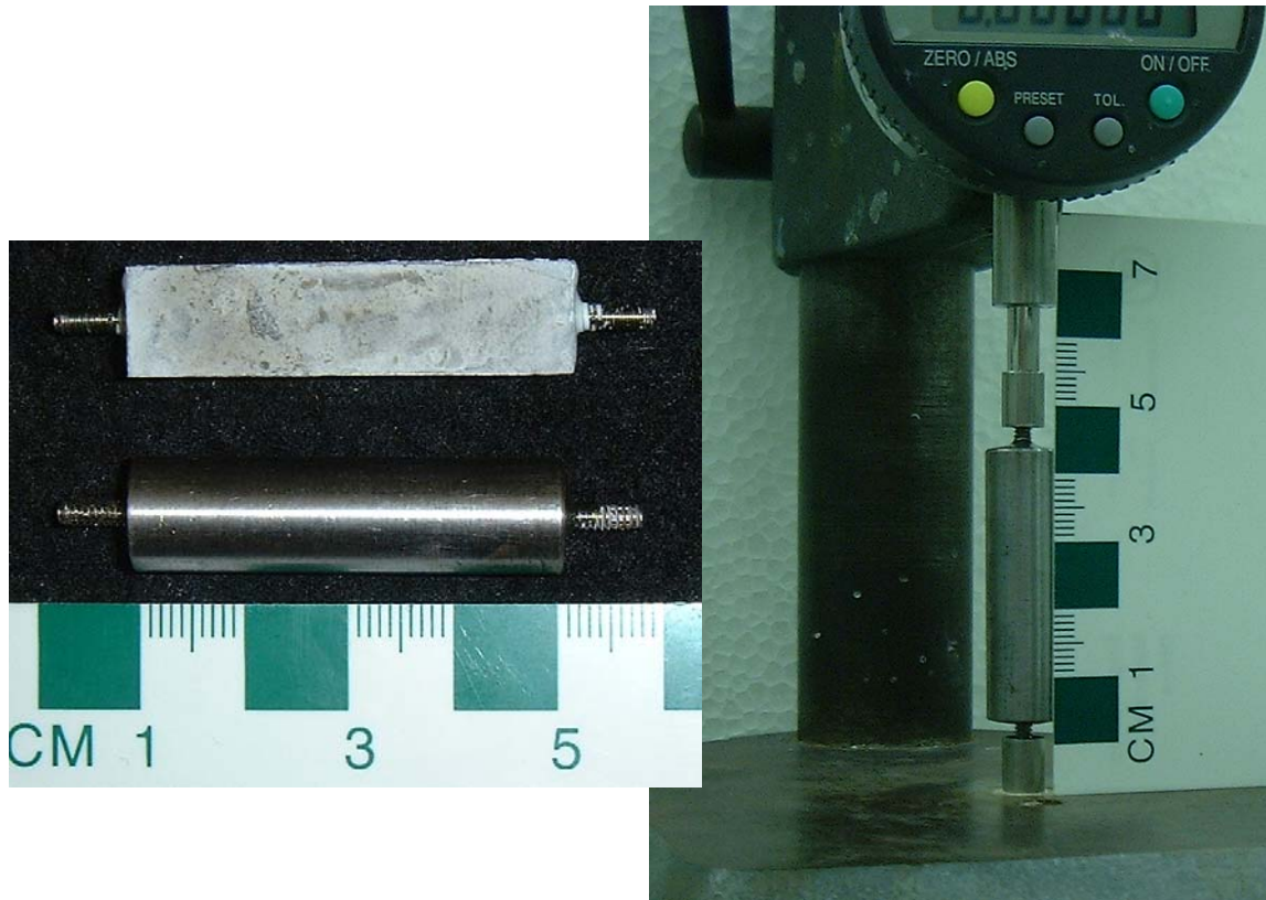
Figure 37: Expansion measurement: A) reference and a specimen, B) comparator with the reference in place.
