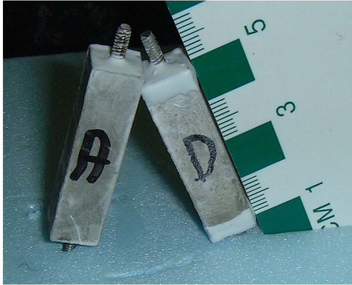
Figure 36: Specimens with epoxy coated ends. Specimen D was also coated 5 mm on the side; Specimen A had only the end sections coated. It was determined that the D-type coating gave more reproducible results [67].
