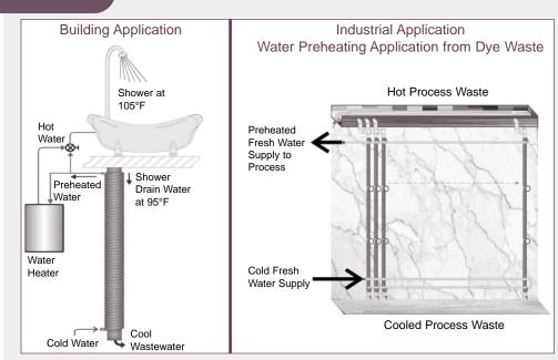
The GFX system, which can be installed on nearly any fluid heat transfer system, saves energy and cuts utility costs for consumers in residential, commercial, and industrial settings.
