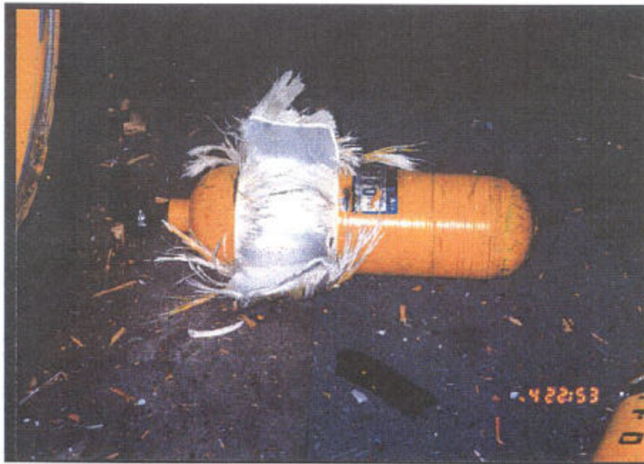
Figure 3. Close-up View of Failed Cylinder after Accident
