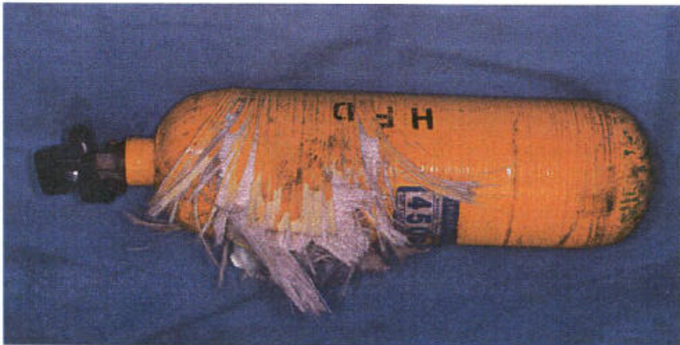
Figure 8. Initial Failure Region of Accident SCBA Cylinder
