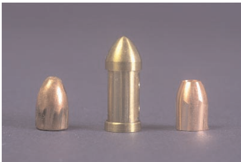
Fig. 2. A master bullet from ATF National Laboratory Center (left), a prototype standard bullet (center), and a SRM 2460 standard bullet (right).
