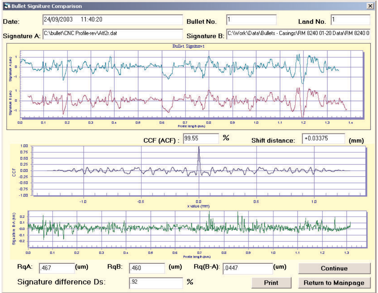
Fig. 3. Bullet signature comparison between the signature of the No. 1 land of S/N 001 SRM 2460 (Signature B, the second profile from the top) and the virtual standard (Signature A, the top profile). The maximum of the cross correlation function CCF_{max} = 99.55\% , the signature difference D_s = 0.92\% . The profile difference of two signatures, B - A , is shown as the bottom profile with different scale.
