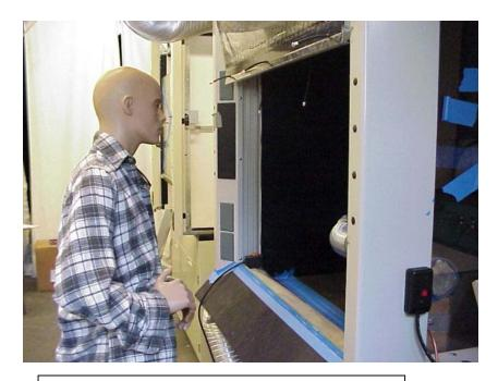
Figure 1: Final Berkeley hood Prototype
