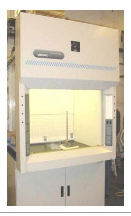
**Fig. 3** – SDSU Berkeley hood containing point-source smoke at LBNL.
