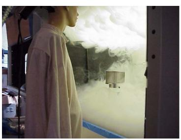
**Fig 8** – Run #1, 50 percent airflow, mannequin at 26 inches above work surface (note ejector).
