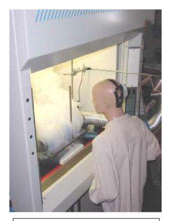
**Fig. 4** – SDSU Berkeley hood containing large-volume-source smoke with mannequin.
