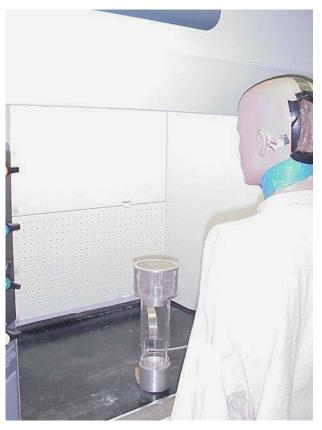
**Fig. 2** – Ejector center position for standard ASHRAE 110 SF6 test.
