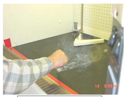
**Fig. 5** – SDSU Berkeley hood demonstrating floor sweep with point-source smoke.
