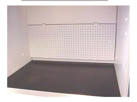
$\label{eq:Fig.6-SDSU} \textbf{Berkeley hood, lower portion of rearbaffle with perforations and slot.}$
