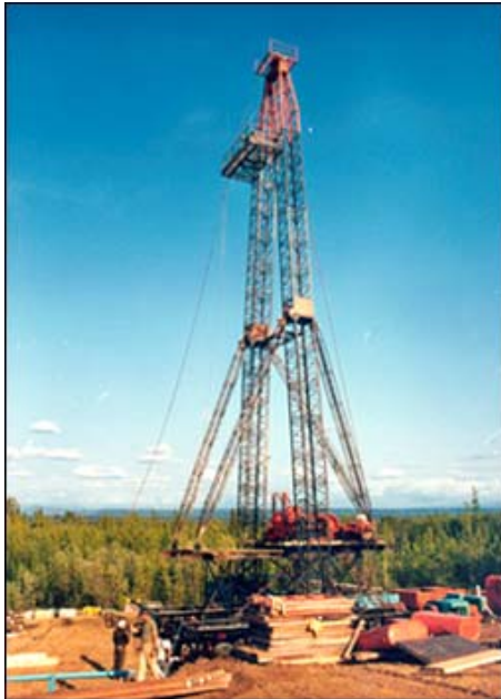
Figure 5. Photograph showing drilling operations at the ARCO Totek Hills Well No. 1 (Map No. 64), about 120 km southwest of Fairbanks, Alaska, 1984. The drilling rig was transported to the site by helicopter. Photographer unknown; photograph provided by Mark McDermott.
