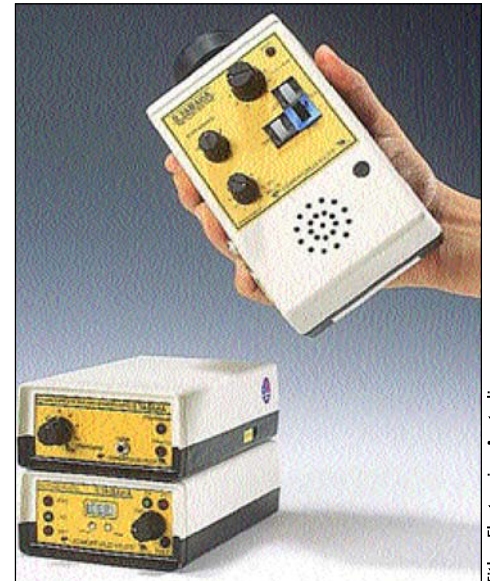
The AnaBat II Detector System was used to record ultrasonic echolocation calls of bats at Pinnacles National Monument.
