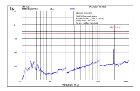
$\label{eq:formula} f < 1~GHz: RBW/VBW: 100~kHz \qquad \qquad f \geq 1GHz: RBW \ / \ VBW \ 1~MHz$  Carrier suppressed with a rejection filter
