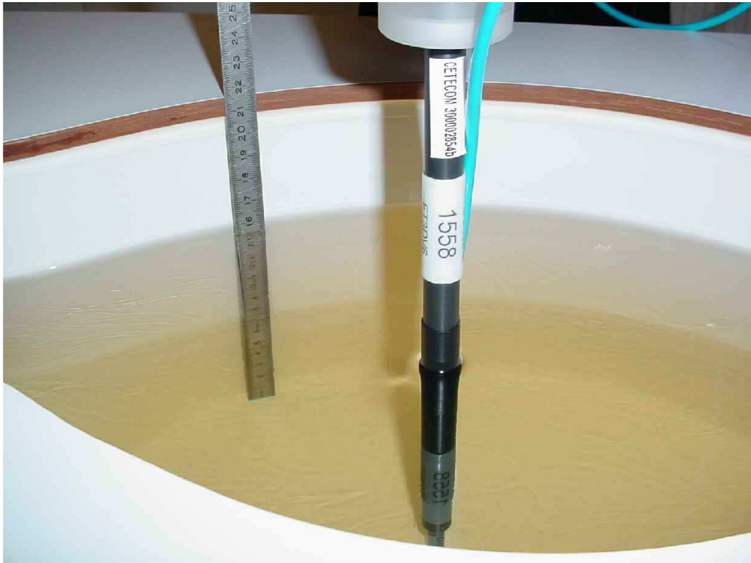
Photo 26: Liquid depth 1900 MHz body simulating liquid
