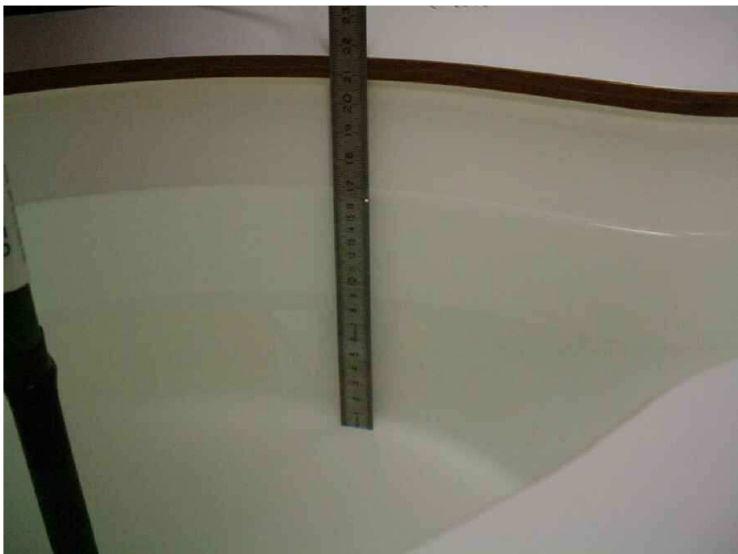
Photo 26: Liquid depth 1900 MHz body simulating liquid
