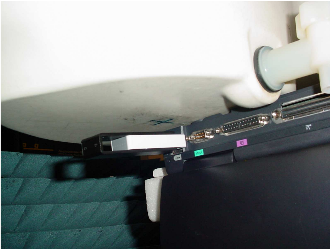
Photo 24: Test position underside with DELL PP01X (11 mm distance of DUT to SAM)
