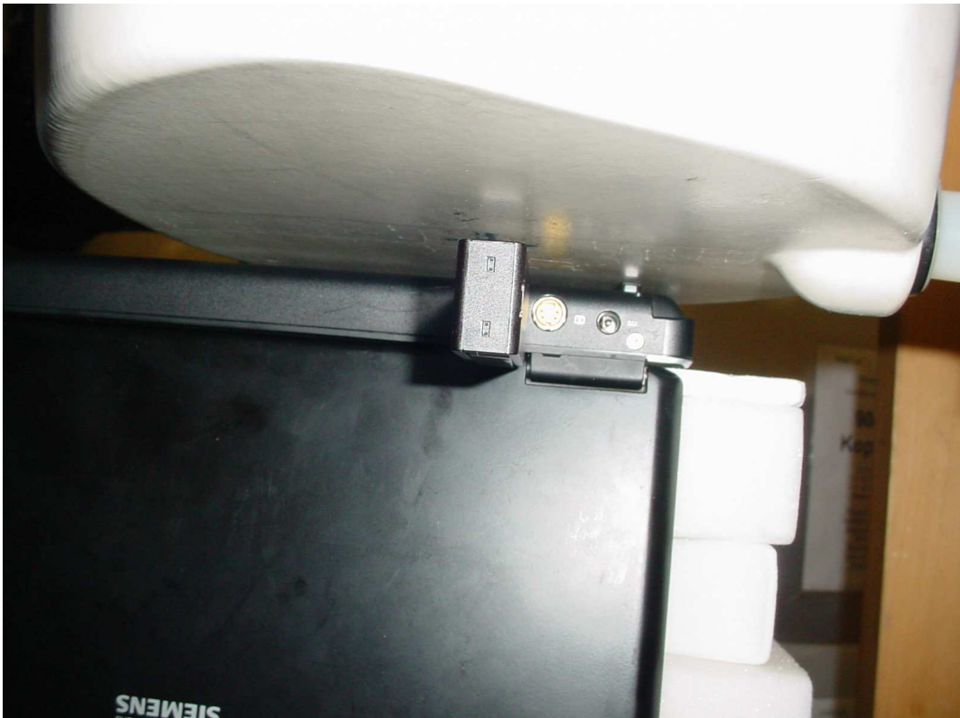
Photo 22: Test position underside with Fujitsu-Siemens (5 mm distance of DUT to SAM)
