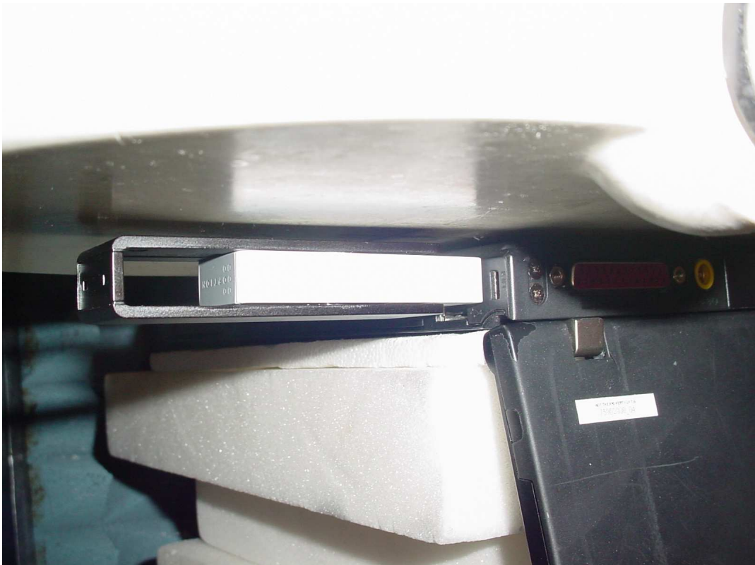
Photo 20: Test position underside with IBM 2372 (2 mm distance of DUT to SAM)
