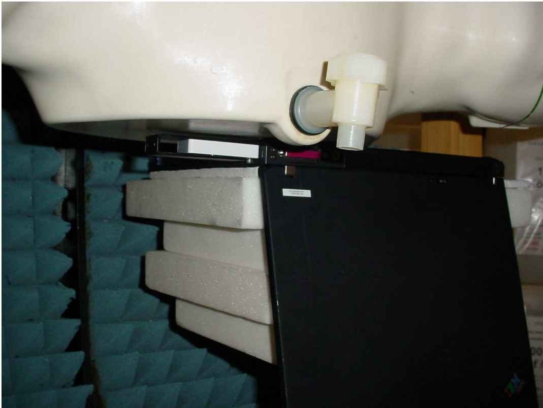
Photo 20: Test position underside with IBM 2372 (2 mm distance of DUT to SAM)
