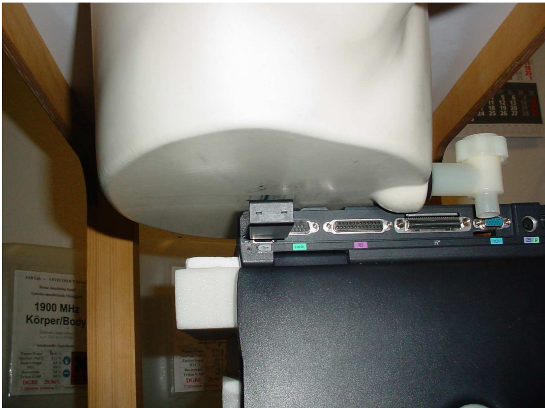
Photo 24: Test position underside with DELL PP01X (11 mm distance of DUT to SAM)
