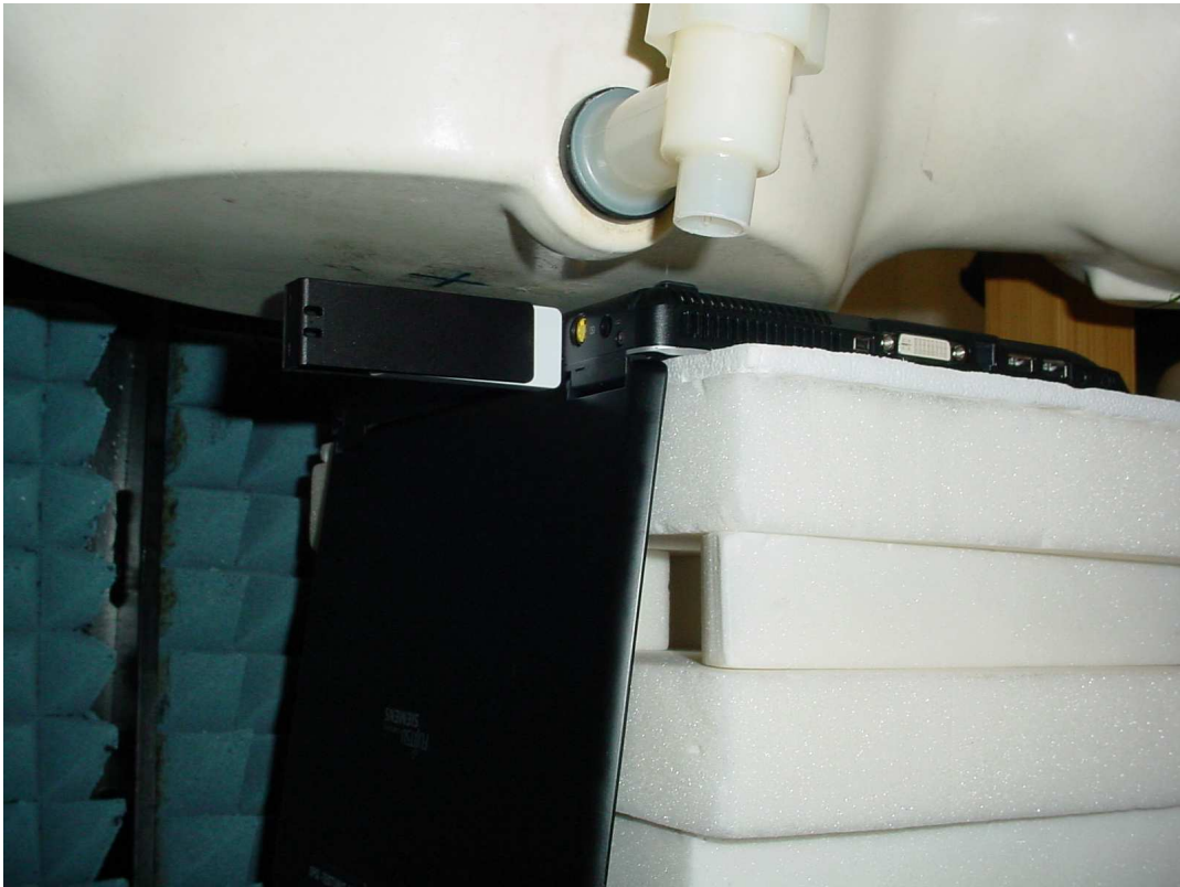
Photo 22: Test position underside with Fujitsu-Siemens (5 mm distance of DUT to SAM)
