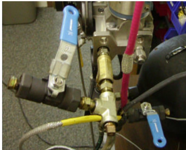
Figure 8: Photograph of OASC installed on PAMP. Each of the blue handled valves is an OASC with a different frequency-pressure curve.
