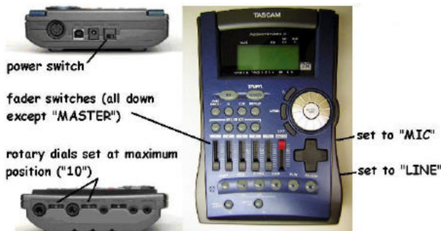
Figure 19: Setting the switches on the TASCAM PS-5.
