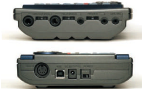
Figures 6 & 7: The Teac TASCAM PS-5 with audio inputs and outputs on the top. On the bottom are MIDI In, USB, and AC-adaptor ports. Selector switches and the Compact Flash port are on the unit's right side. (Broderson, S., 2003)
