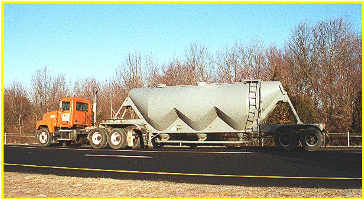
Figure 5B: Conventional Suspension, Bulk Hauler (Class 9) Vehicle Used During First Calibration, October 1998
