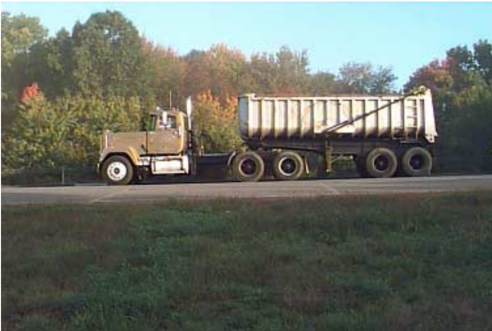
Figure 9B, Conventional Suspension Class 9 Vehicle Used During Third Calibration, October 1999
