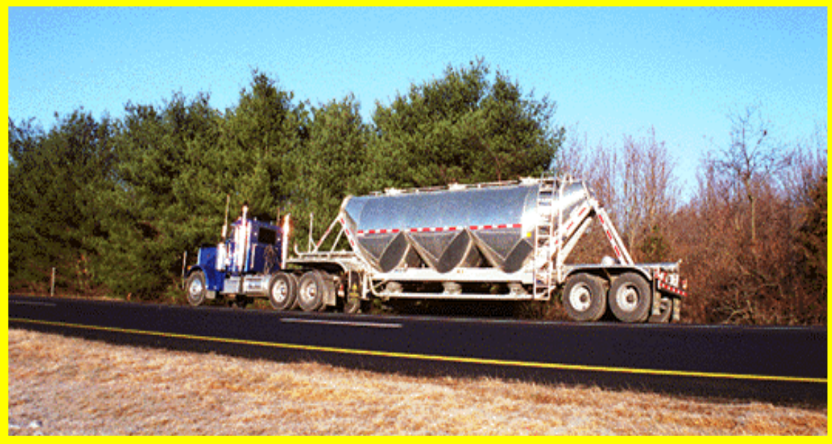
Figure 5A: Air Ride Suspension, Bulk Hauler (Class 9) Vehicle Used During First Calibration, Oct. 1998
