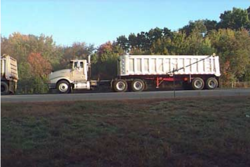
Figure 9A, Air Ride Suspension Class 9 Vehicle Used During Third Calibration, October 1999
