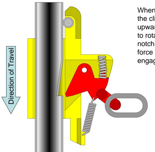
When descending past a rail notch, the climber must apply an outward or upward force on the snap hook link to rotate the pawl away from the notch. They must then release the force after passing the notch to reengage the system.
