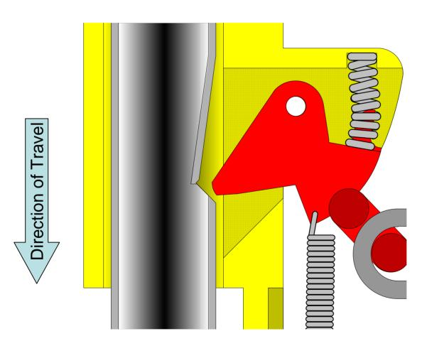
If the notch or pawl becomes damaged or worn during use, the pawl may not catch in the notch. This would increase the fall distance and may result in severe user injury.
