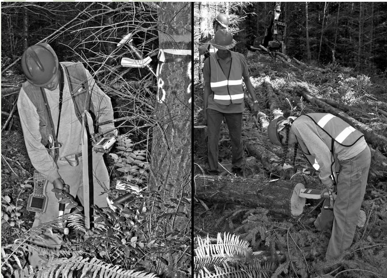
Measuring acoustic velocity in left, a Douglas-fir tree, and right, a Douglas-fir log. Photos: Stand Management Cooperative.
