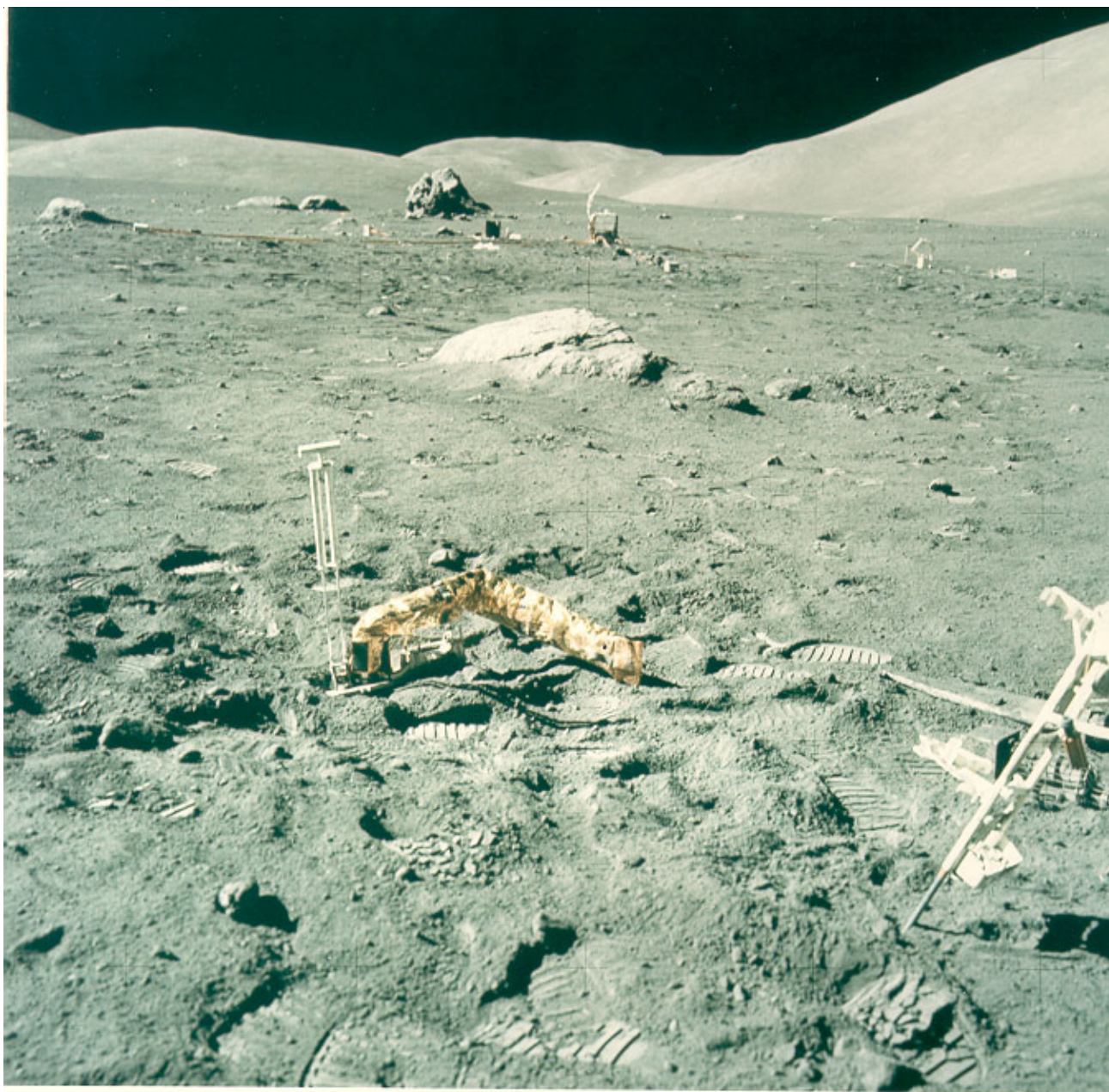
Figure 1: There are no photos of the crew taking the Apollo 17 deep drill core, but this photo of the site, with the neutron probe in place, shows the effort that must have been expended to obtain the three (3) meter deep drill core. AS17-134-20505. The ALSEP site is just beyond.
