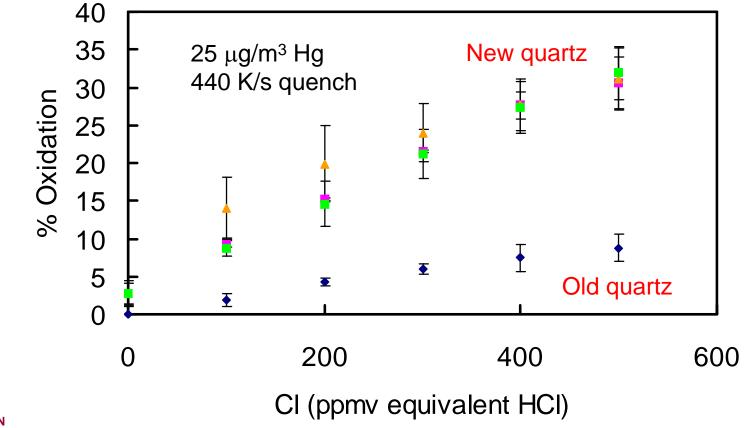
REACTION ENGINEERIng // INTERNATIONAL Experimental – Homogeneous Oxidation
