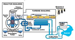
Water is heated through the controlled splitting of uranium atoms in the reactor core and turns to steam. Pumps force the water through the reactor at top speed, maximizing steam production. Steam drives the turbines that turn the generator to make electricity. Cooling water drawn from the river condenses the steam back into water. The water is discharged directly back to the river, reused in the plant, or cooled first in the cooling tower before discharge or reuse.
