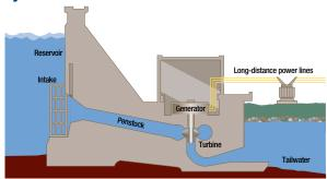
Water from the reservoir rushes through the penstock into the powerhouse. The water spins the turbine, which drives the generator. Inside the generator is a large electromagnet that spins within a coil of wire, producing electricity.
