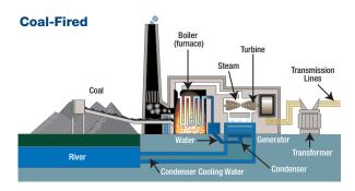
Coal burned in the boiler heats water to produce steam. The steam spins the turbine, which drives the generator. Several TVA coal plants include equipment called scrubbers to reduce sulfur dioxide emissions, and all have some form of controls to reduce nitrogen oxides (not depicted in this diagram).
