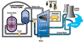
Water is heated by splitting uranium atoms in the reactor core, then held under high pressure to keep it from boiling. It produces steam by transferring heat to a secondary water source, and the steam is used to generate electricity. As in a boiling water reactor, river water condenses the steam and is then discharged back to the river, reused, or cooled in the tower.
