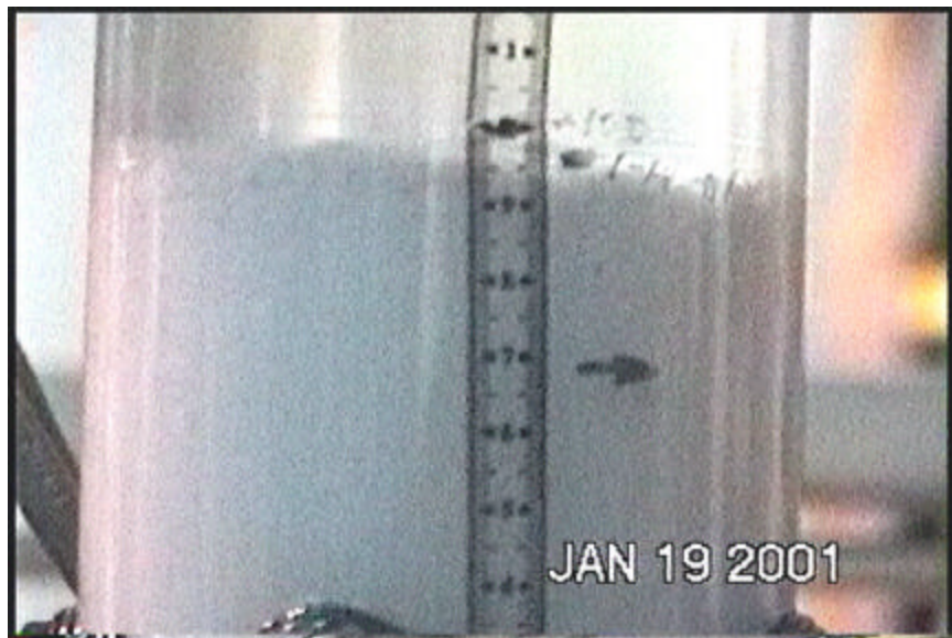
Fig. 4.17. CST bed of downstream column during Mode A at 11:40, 1/19/01.
