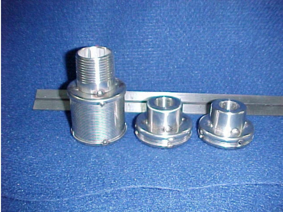
Fig. 3.3. Standard Johnson screen (left) shown alongside custom 5-slot (center) and 2-slot (right) units.
