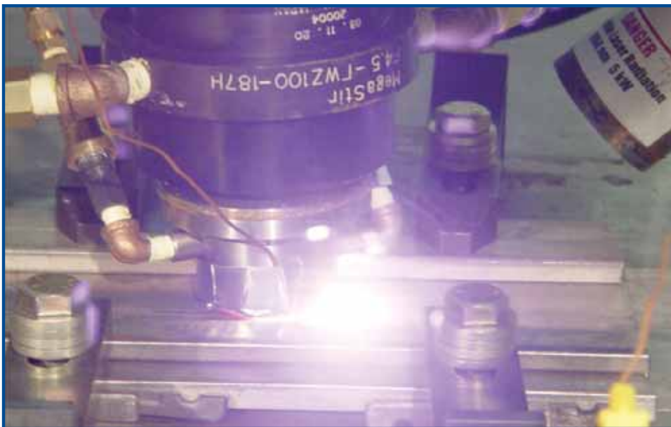
Laser Assisted Friction Stir Welding at Oak Ridge National Laboratory
