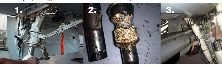
What causes HE in high-strength steel landing gear parts? How about, every @&# thing! Here's a short list: Water (tap and di-ionized), most cleaners on earth (except a tiny handful), rust strippers, every electroplating solution, hoof and mouth disease disinfectants, soft drinks, etc., etc. When steel landing gear parts are exposed to any fluid except authorized cleaning fluids (such as P-D-680), our engineers are programmed to suspect HE and react accordingly.
