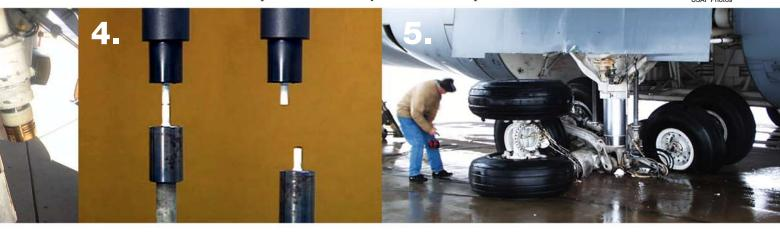
in and day out, in flight or parked. They include stresses to support aircraft weight while parked, stresses due to internal nitrogen pressure, and residual stresses created during initial manufacturing or operational damage. Because landing gear structures support aircraft weight most of the time, they are SCC factories!
