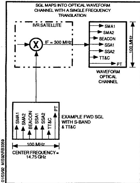
Figure 8: Waveform Forward Crosslink
