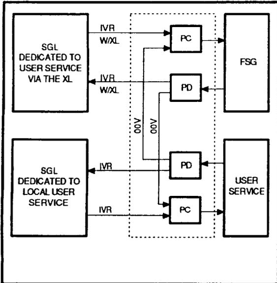
Figure 6: Example Switch Implementation with Dedicated SGL Channels for S-Band Services
