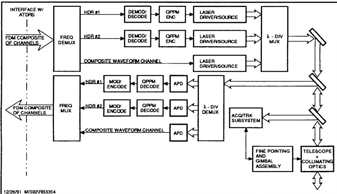
Figure 11: Optical Transceiver Payload for FSG
