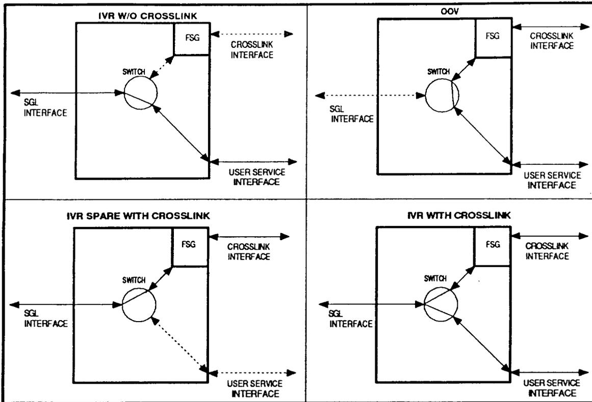
Figure 4: FSG Channel Routing Requirements in All Configurations
