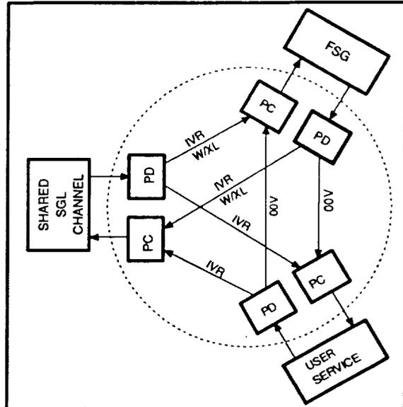
Figure 7: Example Switch Implementation with Shared SGL Channels
