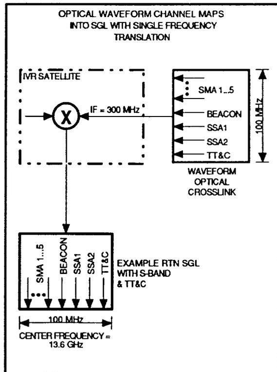
Figure 9: Waveform Return Crosslink
