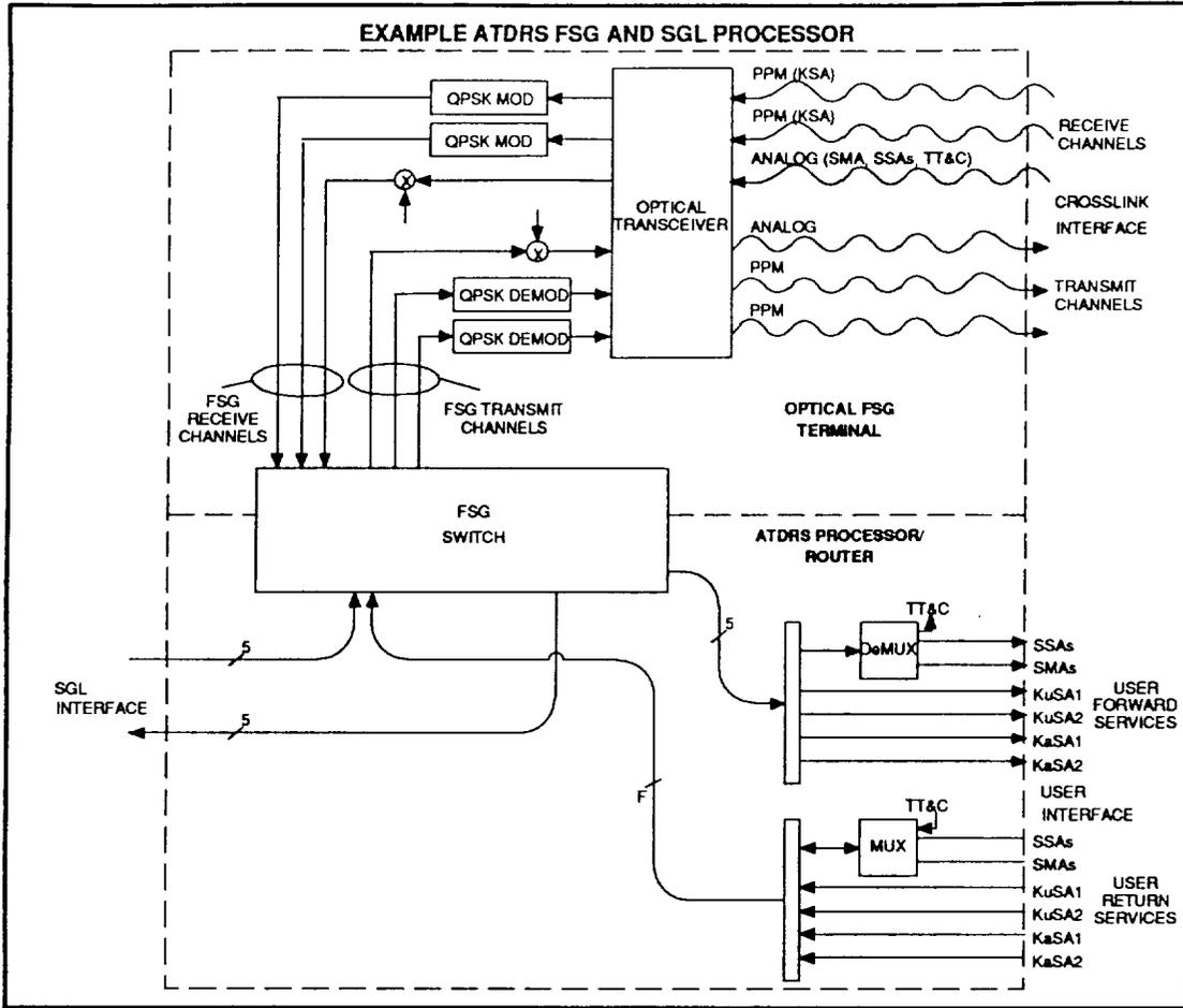
Figure 10: Overview of the FSG Payload
