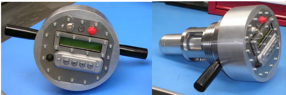
Figure 26. Test equipment used for field debugging, including TDR
