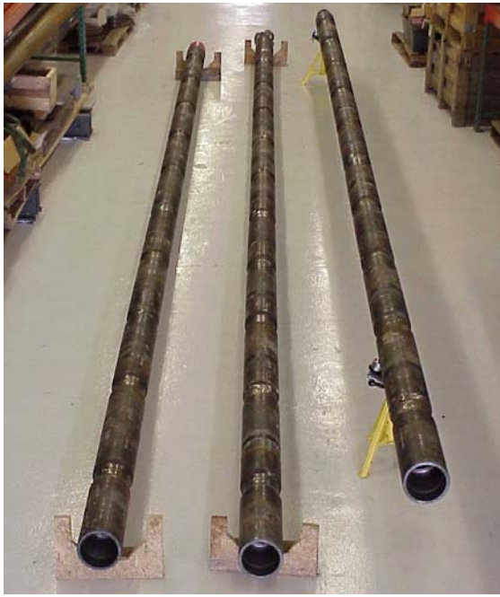
Figure 42. Prototype 5-7/8" XT57 "Joints" used in drilling laboratory testing
