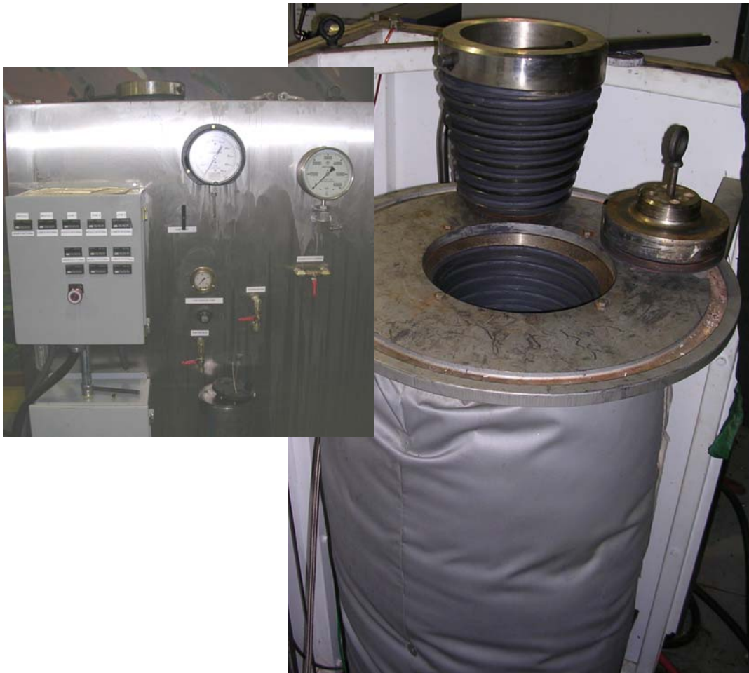
Figure 23. Large HTHP test vessel
