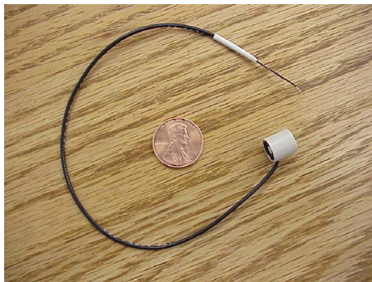
Figure 1. Acoustic Transducer used in early development efforts
