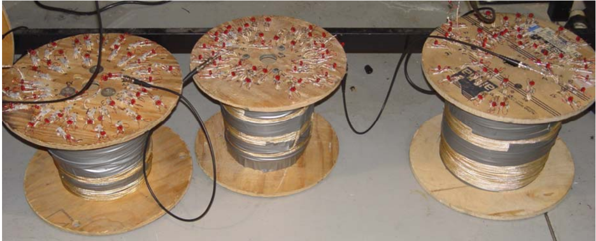
Figure 19. Compact physical model - simulation of 1 mile of drill pipe
