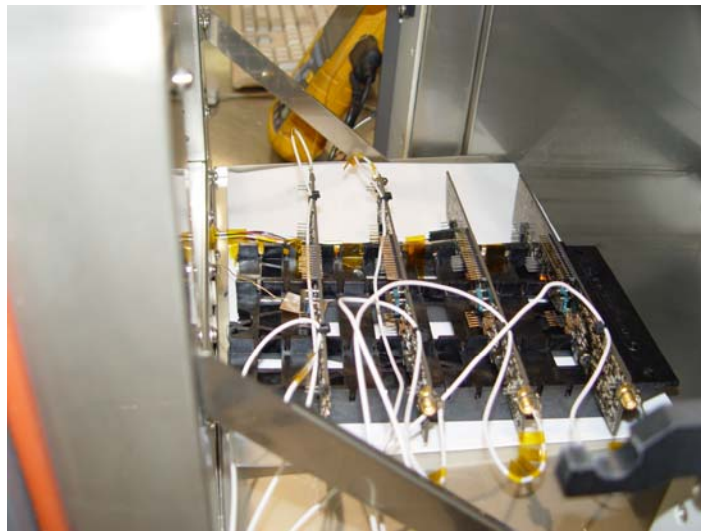
Figure 36. Printed Circuit Boards operating inside the Test Chamber
