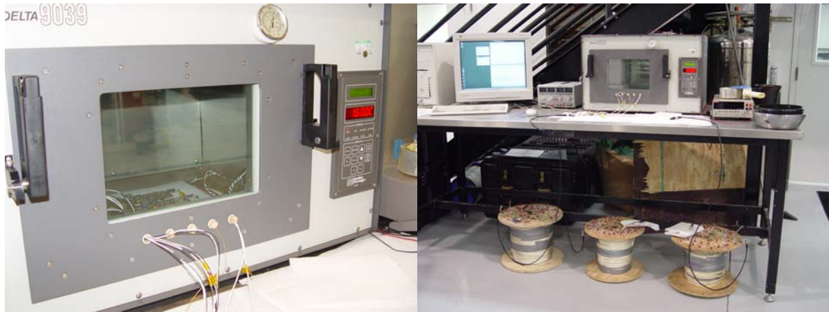
Figure 35. Oven qualification of circuit boards through simulated transmission line
