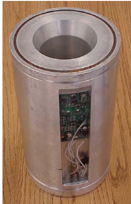
Figure 43. Rudimentary Smart Bit Prototype
