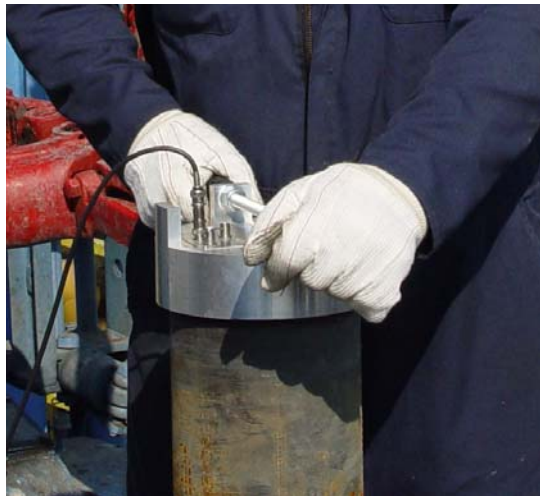
Figure 48. Portable sub for connecting the network during Tripping
