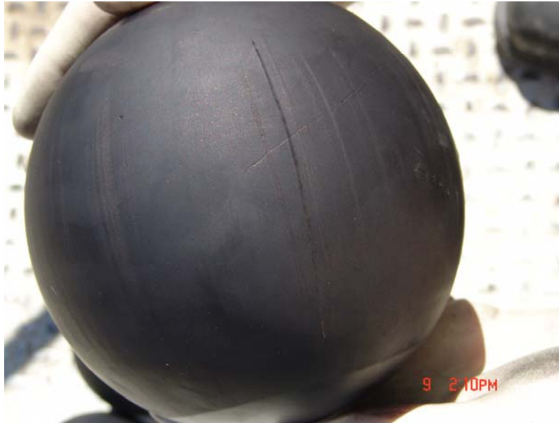
Figure 33. Damage to Hard Rubber Wiper Ball
