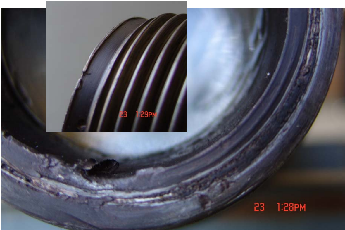
Figure 50. Stabbing Damage to Data Swivel
