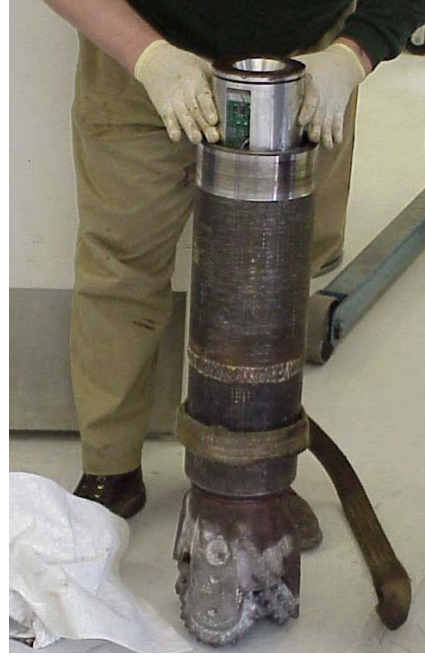
Figure 43. Rudimentary Smart Bit Prototype
