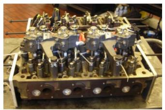
Electro-hydraulic Intake Valve System control installed on the Navistar 6.4 L V8 engine.
