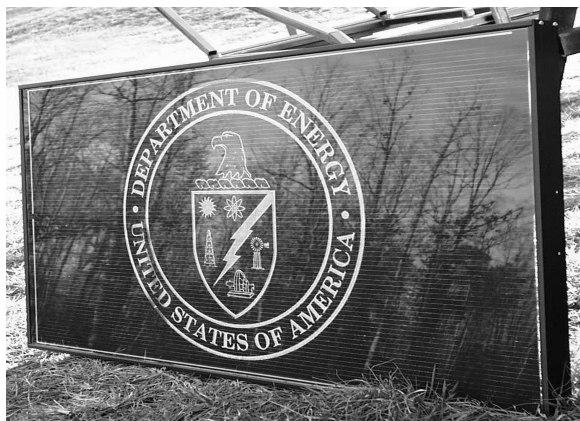
Figure 2: Prototype BP Solarex PowerView, an insulated viewglass window developed in PV:BONUS2.
