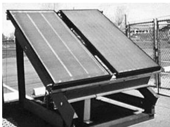
Figure 4: Prototype Phototherm product adjacent to thermal-only collector on test.
