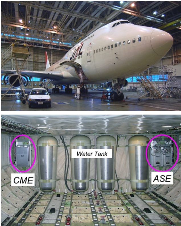
Figure 6. Forward cargo compartment of Boeing 747-400. ASE and CME are installed beside the water tanks in the forward cargo compartment.
