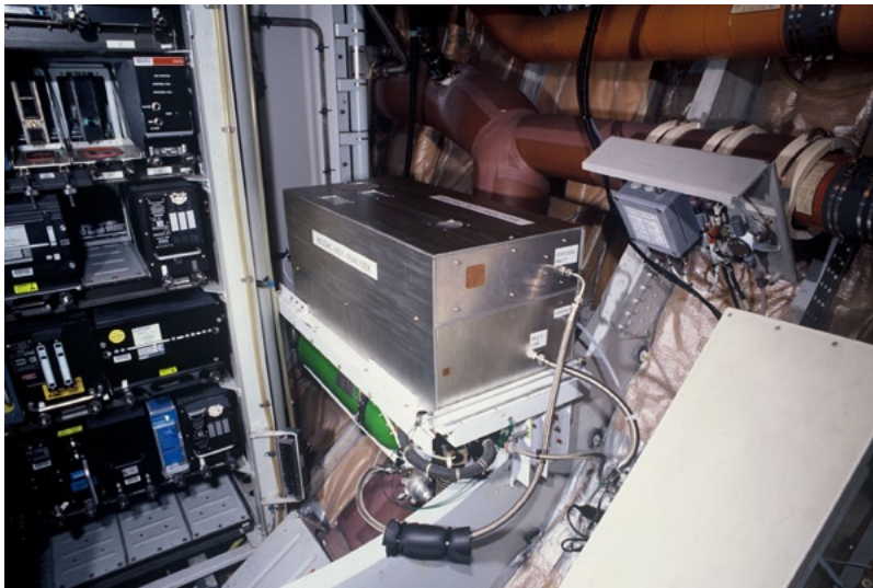
Figure 1. The MOZAIC NO y instrument in the avionics bay of a Lufthansa A340-300. The new IAGOS equipment will be installed at this location (see Fig. 2 for details). Photo: Udo Kröner, Deutsche Lufthansa.
