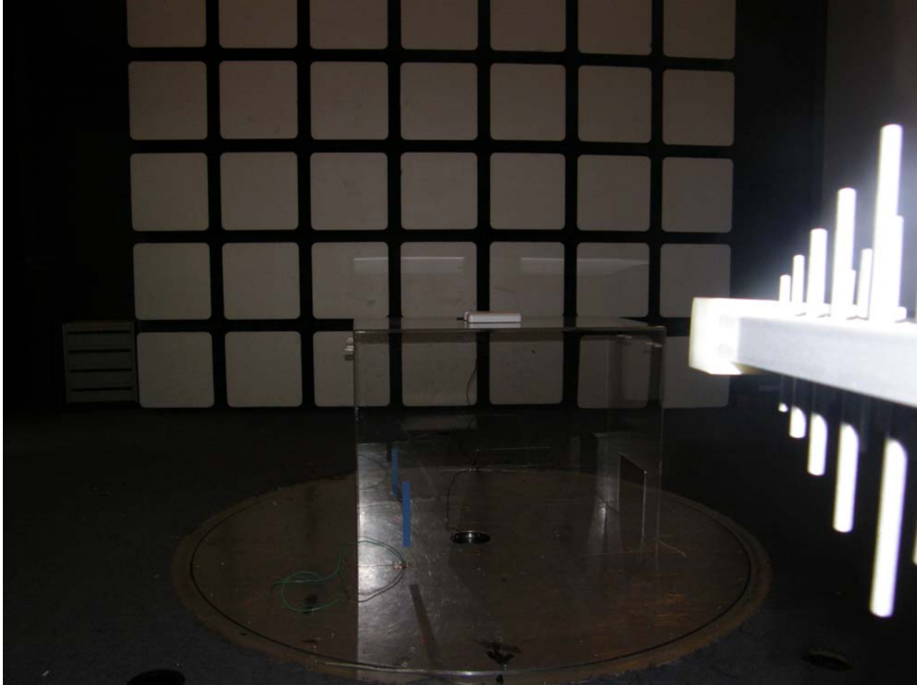
Photograph 2. Radiated Emission Limits Test Setup
