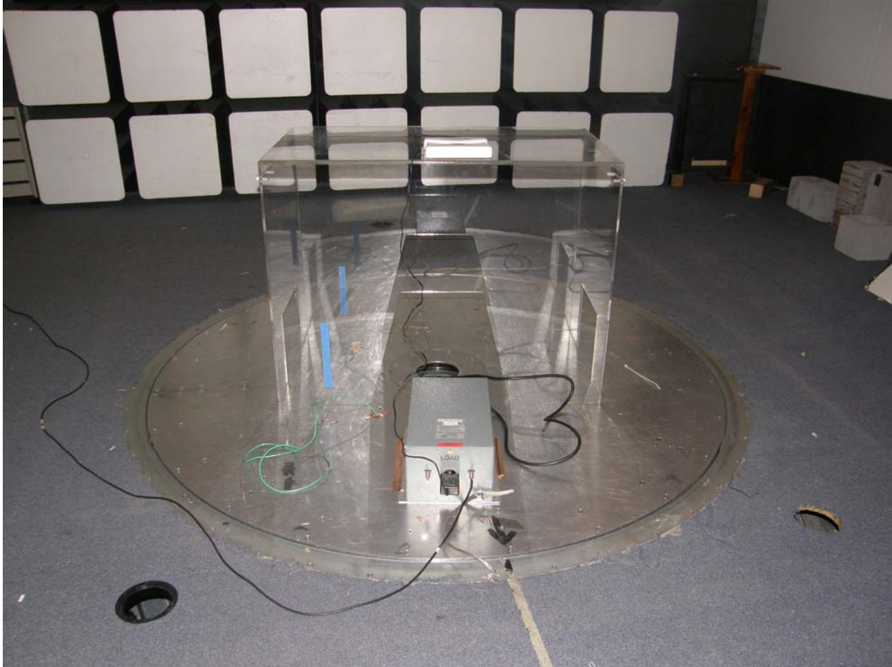
Photograph 1. Conducted Emissions Test Setup
