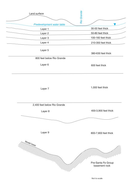
Figure 3. Configuration of layers in the model. Modified from McAda and Barroll (2002, fig. 8).
