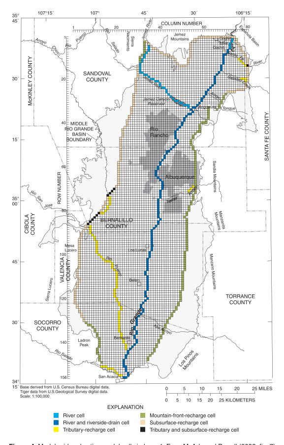
Figure 4. Model grid and active model cells in layer 1. From McAda and Barroll (2002, fig. 7).
