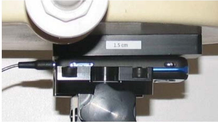
Photo of the device positioned for Body SAR measurement. The spacer was removed for the tests.
