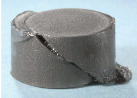
FIGURE 5. PHOTOGRAPH OF Ti-6Al-4V SAMPLE AFTER TESTING IN COMPRESSION
