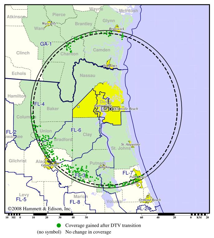
CP (solid): 1000 kW ERP at 288 m HAAT vs. Analog (dashed): 3310 kW ERP at 289 m HAAT
