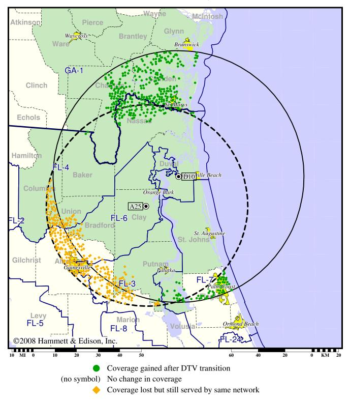
CP (solid): 790 kW ERP at 417 m HAAT vs. Analog (dashed): 2630 kW ERP at 311 m HAAT
