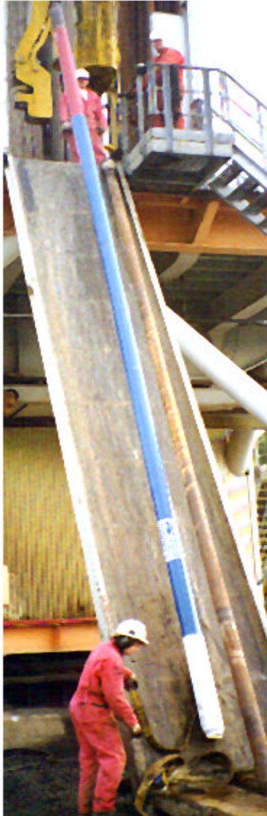
Figure 3. DHP Being Picked Up on the Drill Rig in Norway.
