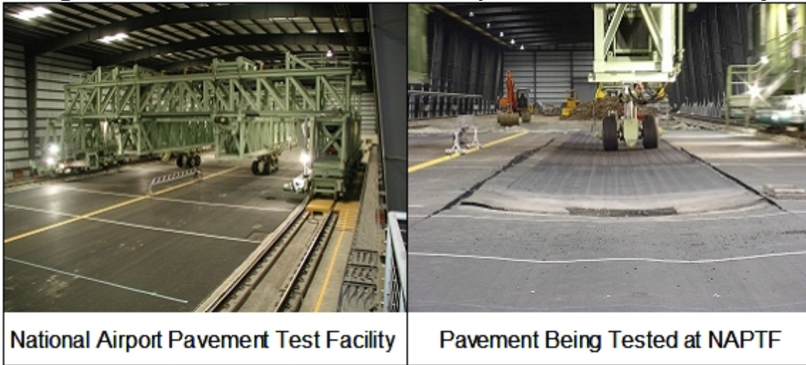
Figure 15: Illustration of the National Airport Pavement Test Facility
