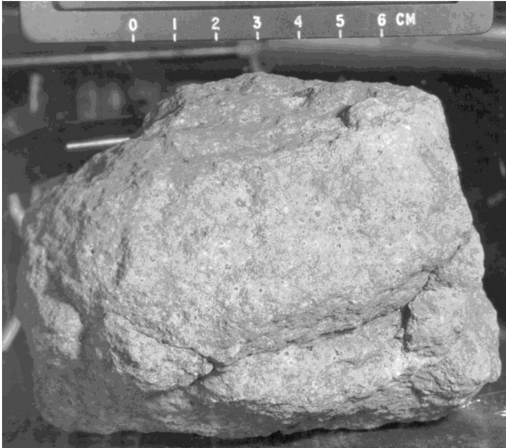
Figure 1: Photo of 12065 showing numerous zap pits on rounded surface. Scale is in cm. NASA # S69-60591.
