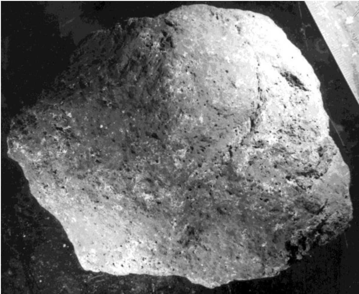
Figure 2: Original photo of rounded, dust-covered, surface of 10017,0. NASA S69-47573. Note micrometeorite craters and vesicles. This was originally thought to be the “top” surface until 56Co was found on the other side (figure 3).
