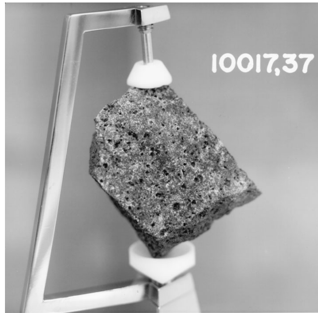
Figure 20: Photo of display sample 10017,37 showing micrometeorite craters and vesicles. NASA photo #S84-40064.
